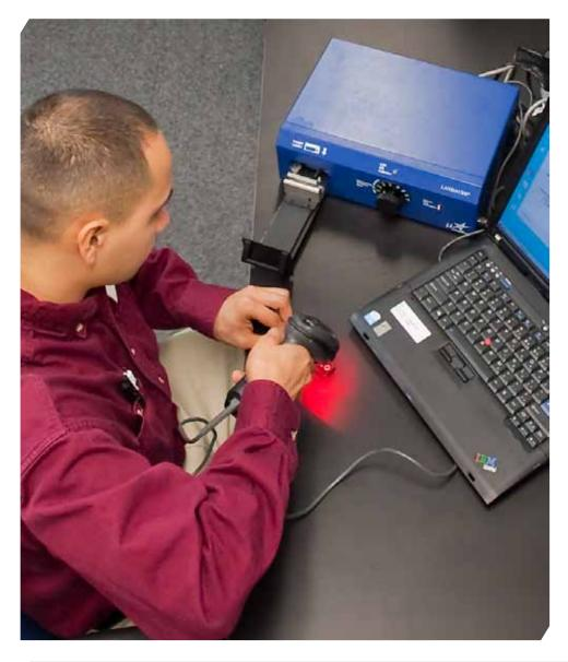
The microStar reader is a compact, lightweight, portable reader that can be taken anywhere immediate results are required. It uses aluminum oxide (AI<sub>2</sub>O<sub>3</sub>) detectors to measure radiation exposure and reads the measurement with optically stimulated luminescence (OSL) technology.
